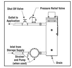
Side Arm — Requirements of large storage tanks can be satisfied by using a number of circulation heaters, providing flexibility in temperature control and reducing power demand.
