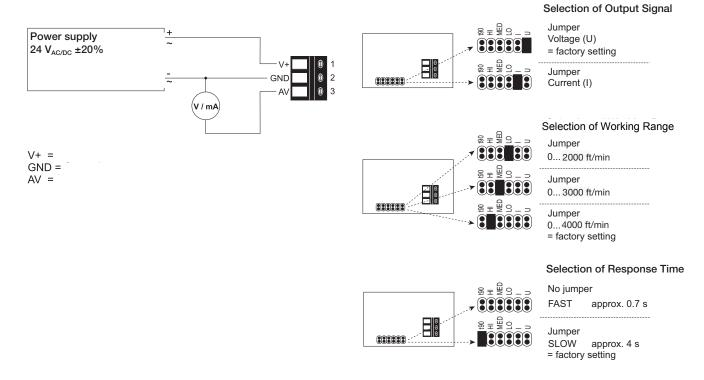
The output signal, working range and response time are selected via the jumpers according to the picture.
