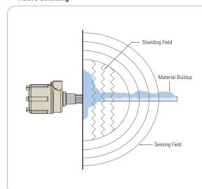
All Ramsey CAP Series level controls feature an active shielding technology to eliminate false readings from material build-up. The shield emits a competing signal which forces the sensing field farther out away from the probe body. This means the sensor is examining a larger area around the probe and is able to look past any material build-up directly on the probe.
