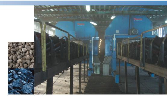
The Thermo Scientific Ramsey Model SWAX-7000 sweep type sampling machine offers an economical, simple means to procure a representative sample directly from a main stream of material. Direct increments are obtained from in-motion, horizontal or inclined conveyors.
