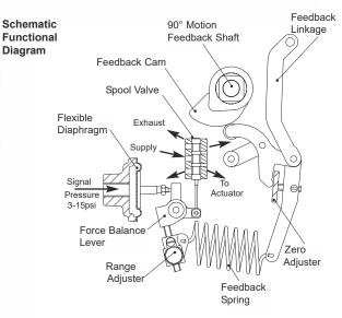
The AP positioner moves an actuator to a position set by a 3-15psi control signal and holds it there. Its features are:
